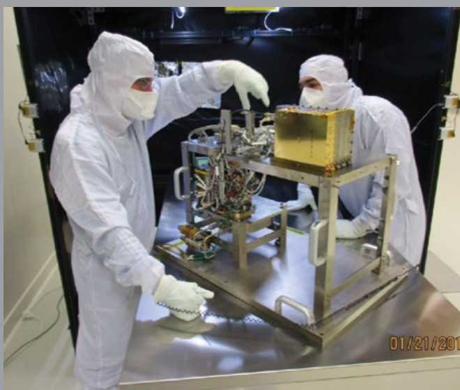
ExoMars 2018 (now 2020) mission: MOMA instrument EQM in integration room before entering the ultraclean facility for integration into the ALD (Thales Alenia Space Italy)
