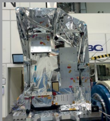
The Structural Thermal Model of the Sentinel-4 Optical Instrument Module at the IABG Test Centre, Munich (OHb)
