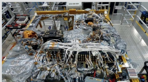
Solar Orbiter service panel Flight Model integration
