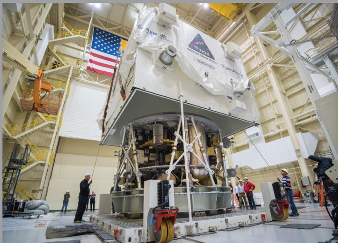
ESA's European Service Module Structural Test Article here being unpacked after transport to NASA Glenn's Plum Brook facility in November for testing in the Space Power Facility in 2016 (NASA)
