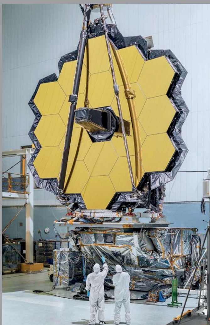
Fully integrated JWST Optical Telescope with the Integrated Science instrument module, ready for the environmental test campaign (NASA)
