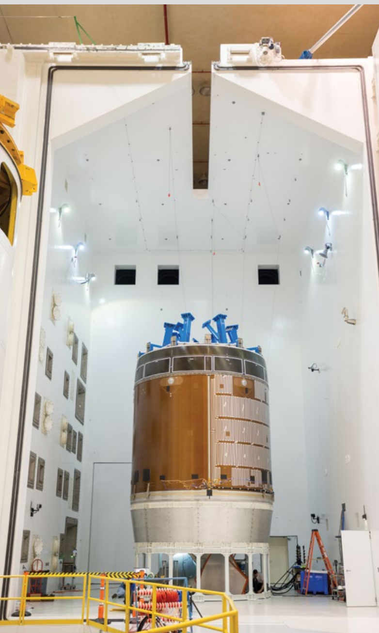
The ESM Structural Test Article being prepared for acoustic and vibration testing at NASA Glenn's Plum Brook facility, Sandusky, Ohio (NASA)
