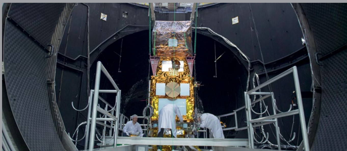
Sentinel-2B entering the Large Space Simulator at ESTEC in June (Airbus D&S)
